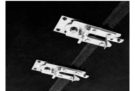
Connect: All chair components ship with high grade, metal ganging brackets installed. The unique design slides together and holds tight until released by simply lifting up on the receiving chair unit. Don't want to gang units together? No problem. Each ganging bracket pivots and folds under to be concealed for later use.
